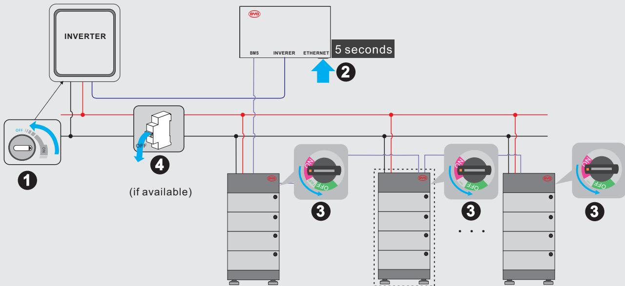
Switch Off Process: ① Inverter; ② BMU; ③ PDU Air Switch; ④ Switch between Battery and Inverter (if available)
