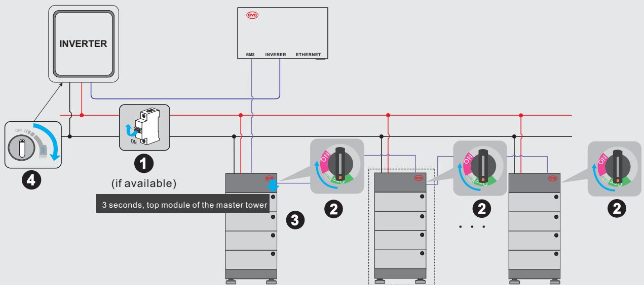
Switch On Process: ① Switch between Battery and Inverter (if available); ② PDU Air Switch ③ Battery; ④ Inverter
