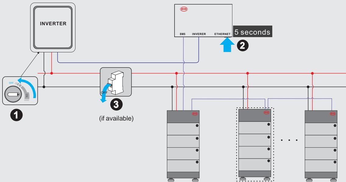
Switch Off Process: ① Inverter; ② BMU ; ③ Switch between Battery and Inverter (if available)
